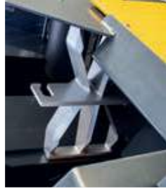
Automatic height adjustment of the knife according to log diameter
