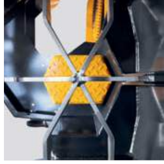
Hydraulically adjustable height of the splitting knife.
