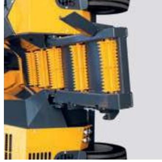
Adjustable hydraulic transport rollers
