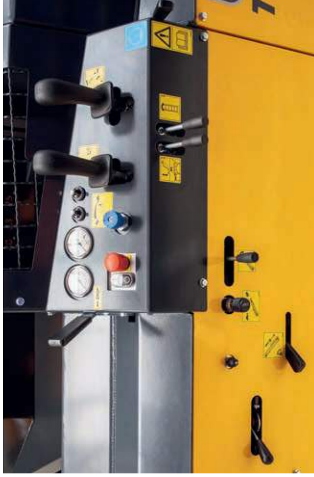
Mechanical control with ergonomically positioned handles
