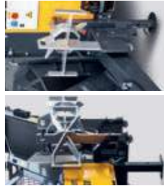
Knife holder for working position and transport position
