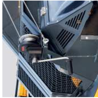
Mechanical winch for tilt adjustment of the conveyor belt
