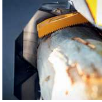
Hydraulic clamp holds log during cutting.
