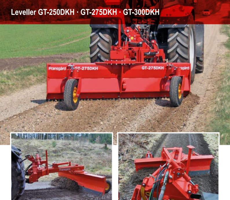
The GT-250DKH/GT-275DKH/GT-300DKH levellers are the top models of Fransgård levellers. They have all the same great advantages as the GT-DK version. Here you get a leveller that always gets down into the road material and easily makes a road slope, so water easily runs off the road.
