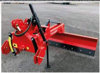
Fransgård's hydraulic GT-250HNZ/GT-275HNZ levellers are used for efficient levelling of soil, clearing of snow and smoothing roads especially in very hilly landscapes and where often only smaller tractors (max. 120 hp.) can be used. The construction is built lighter than our DKH models, but it comes with many of the same features.
