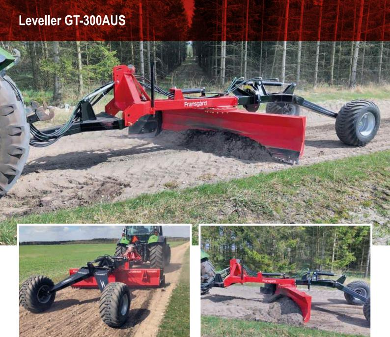
The towed model has the same unique and proven construction as the GT-DKH version. The construction provides a very smooth working process and good possibilities to make a slope on the road so that rainwater always runs away from the road.
