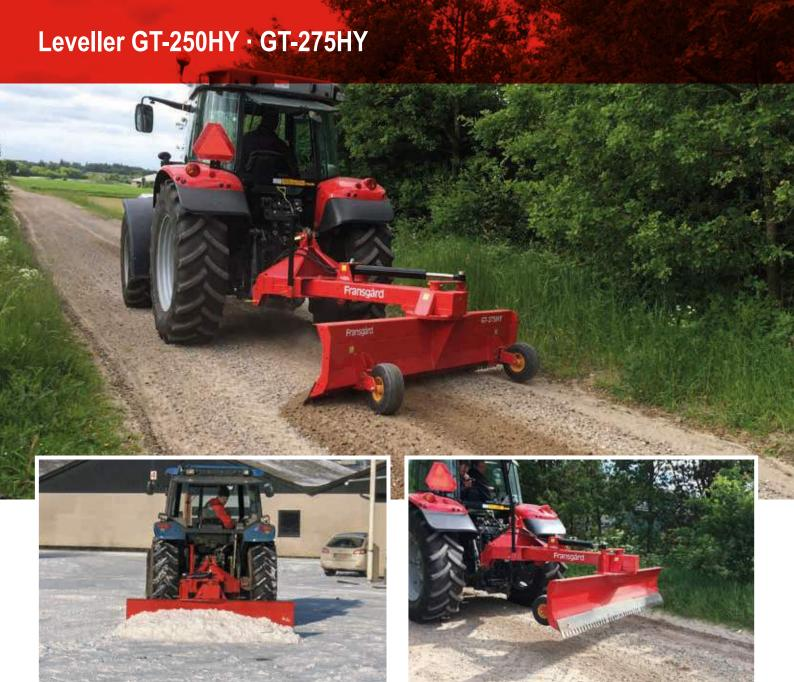
Fransgård's hydraulic (HY) levellers are used for efficient levelling of soil, clearing of snow and smoothing of roads. The leveller has been developed and designed according to know-how accumulated over many years of experience with mechanical levellers. The quality is high as the leveller is Made in Denmark at our own factory in Farsø.
