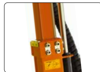
Terminale telescopico con pattini antiusura registrabili. Telescopic extension with adjustable wear plates.
