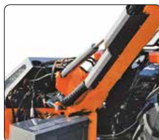
SAB Sistema antiribaltamento. SAB system Roll-over protective kit with inclinometer.
