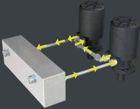
serial oil flow (simplified representation)
