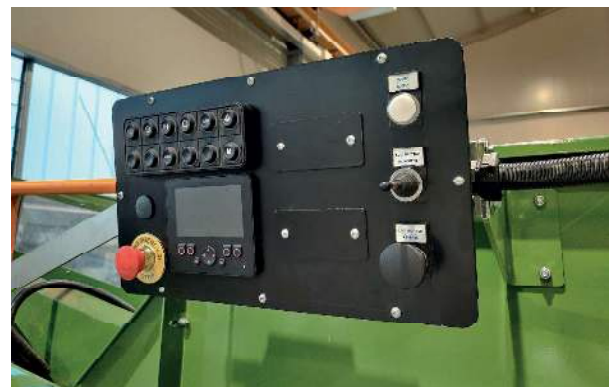
K650 - Control panel
