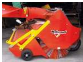
Collecting box, mechanical emptying
