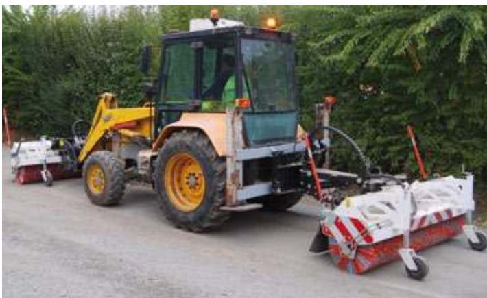
Setraclean - Mounting on backhoe loader with rear SETRA plate + one mounted on the front loader
