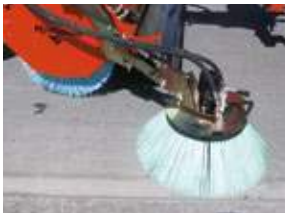
Side brush Ø 700 with rotation reverser
