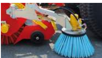
Side brush Ø 550 mm with motor, hoses, 3-way valve (standard version with central brush)
