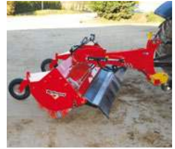
SUPERCHAMPION 2100 A with hydraulic offset and angling
