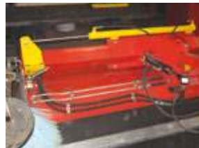
Hydraulic angling by a cylinder and hydraulic offset by motor
