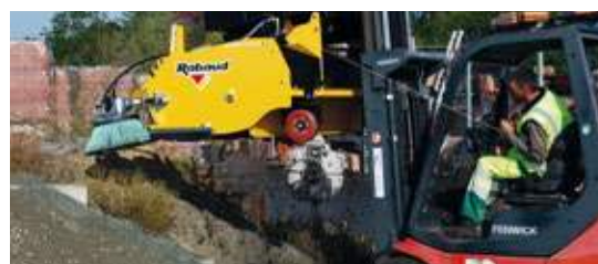
Collecting box emptying from the driver station
