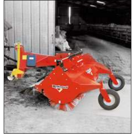
SUPERCHAMPION 2100 A with hydraulic offset and angling
