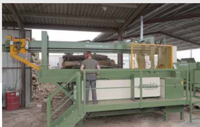
Platform for control board with stairs
