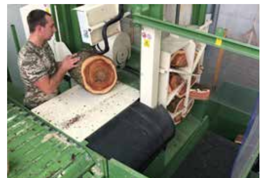
20 Ton splitting station, 2+4+6 folds grid
