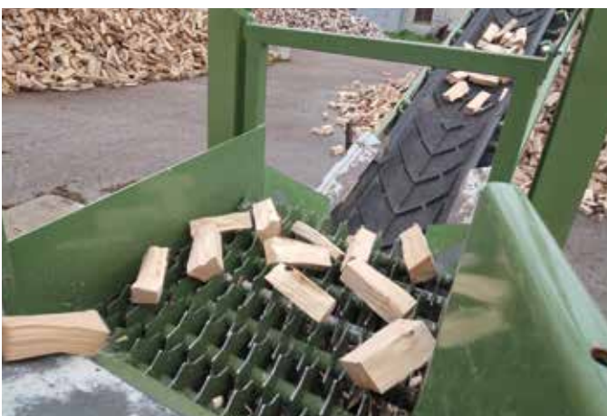
Cleaning rollers for bark and residual sawdust
