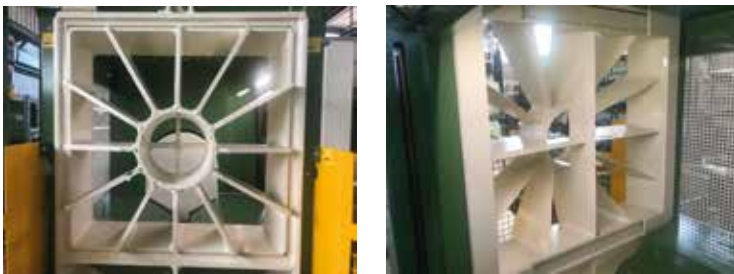
Removable for maintenance operations and interchangeable splitting sector with 10 or 12 or 16 or 18 or 24 folds
