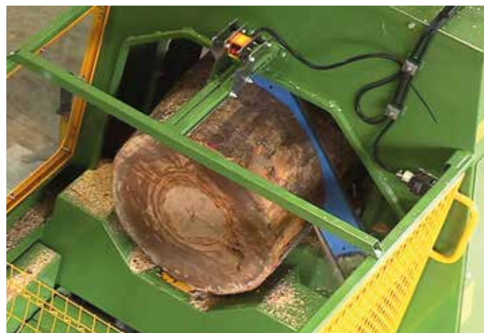
Photocell for automatic log length measurement
