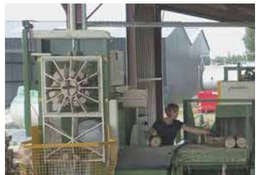
32 Ton splitting station, 2+4+6+16 folds grid
