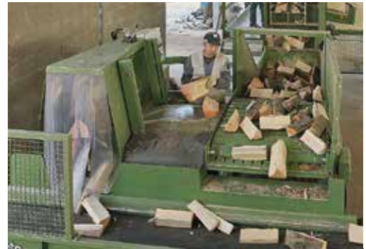
11 Ton splitting station, 2+4 folds grid
