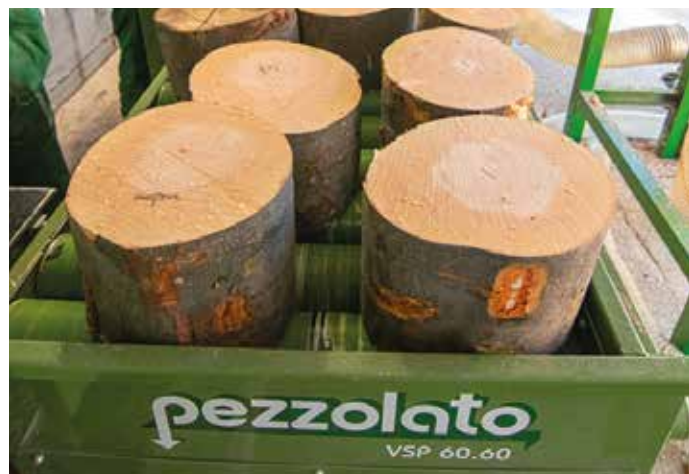
Motorized rollers table for transferring cut logs
