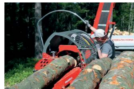
The machine's direct drive hydraulics enable simultaneous functions with effortless motions of the operating lever.
