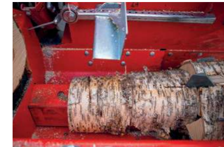
38 Pro has a halfstroke function for making the splitting process of short firewood faster. The half-stroke splitting can be easily controlled with a button in the front panel.
