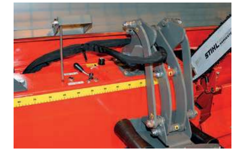
The AC 10 automatic chain tensioner maintains optimal saw chain tension at all times. The chain can be conveniently replaced after releasing chain tension with the lever pictured – no tools required!
