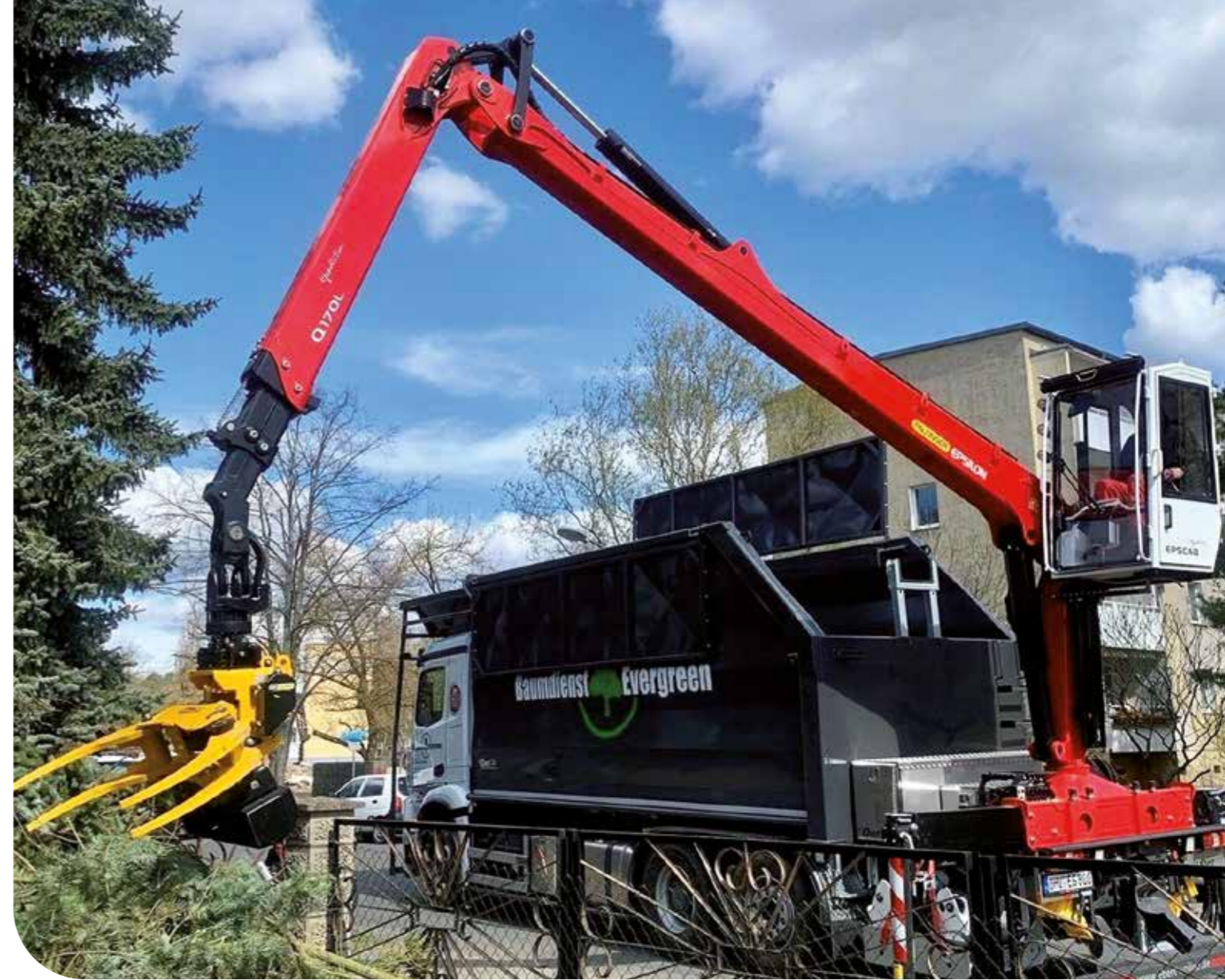
Truck with a GMT050 grapple saw and GMT C10 quick coupler system
