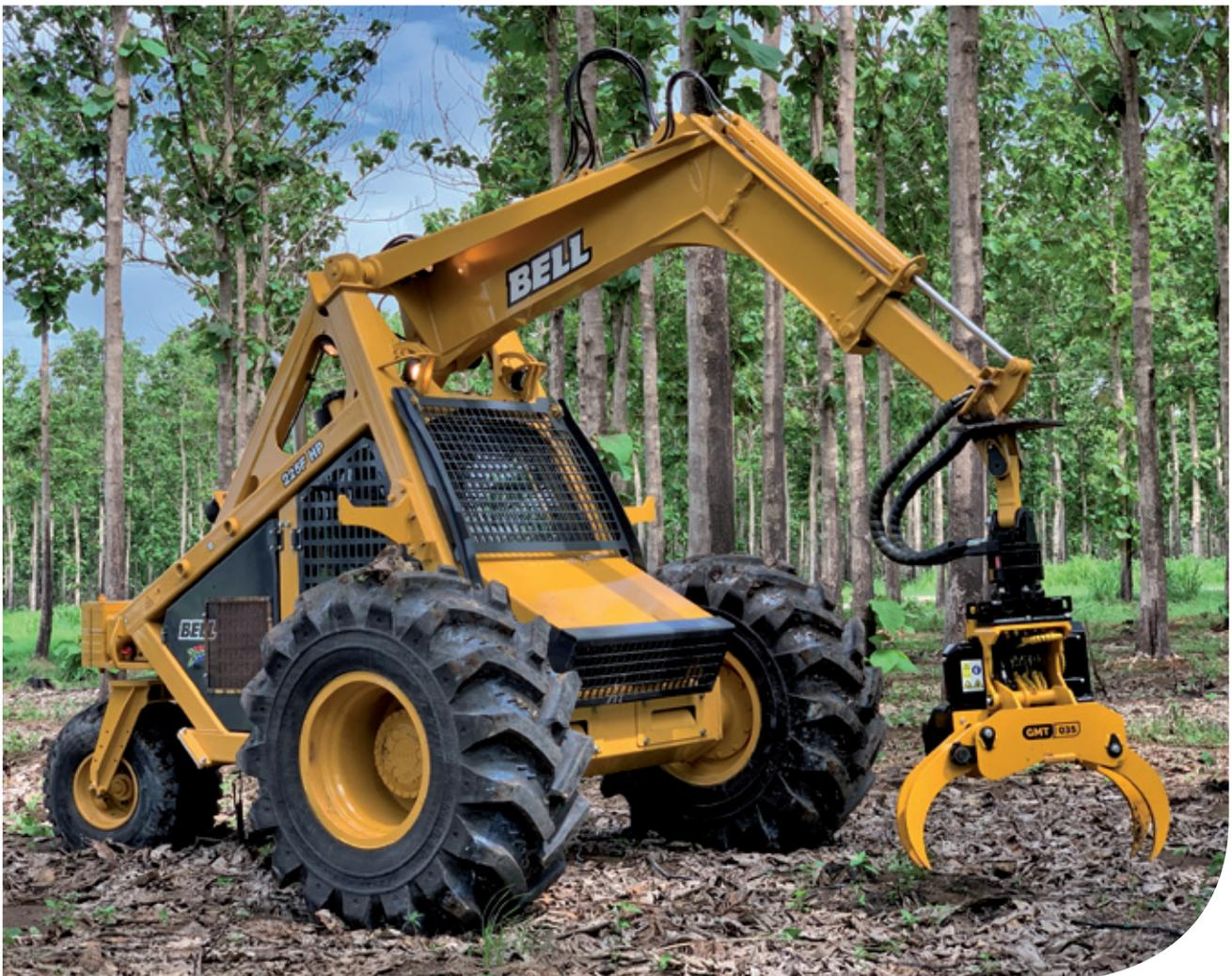
Bell Equipment logger with a GMT C10 quick coupler and GMT035 grapple saw
