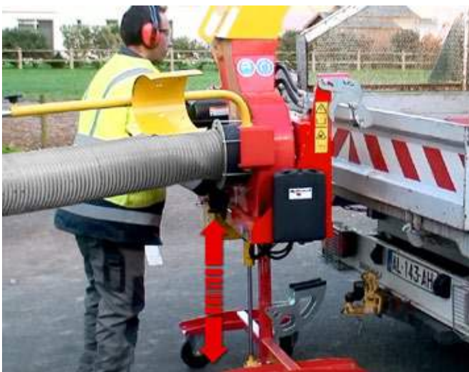
Hydraulic set-up at the rear of the truck – One operator needed
