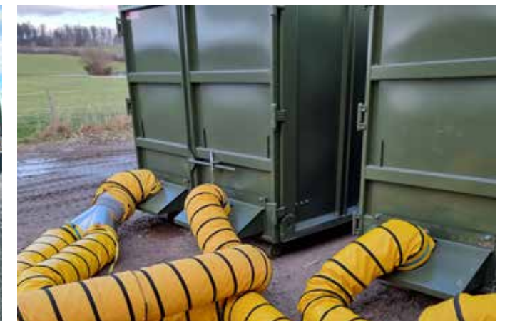
Heat distribution made easy. The drying air enters the drying container effortlessly via warm air hoses.
